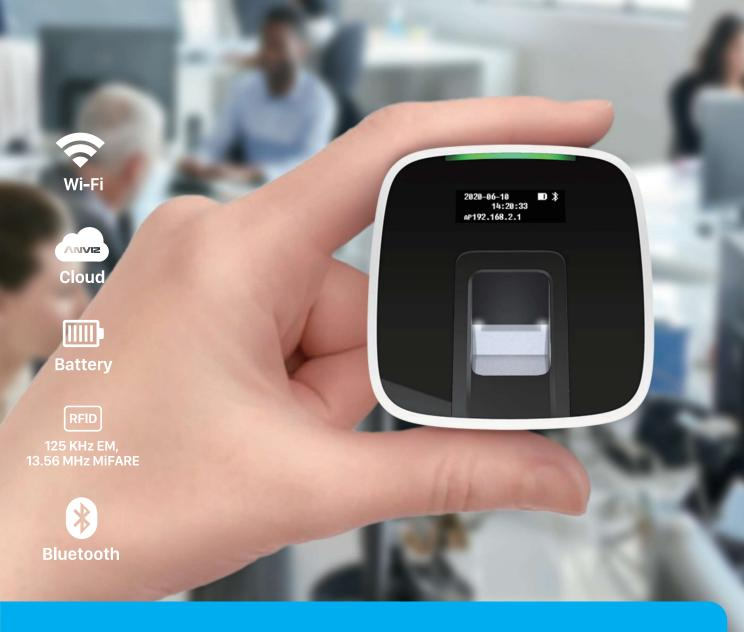
M-bio is a portable fingerprint and RFID Time & Attendance terminal featuring Anviz next generation AFOS touch active fingerprint sensor and rechargeable Li-ion Battery. Standard with Wi-Fi and Bluetooth function, supports CrossChex Cloud and CrossChex Mobile APP. Meanwhile, the M-bio based on embedded Linux system platform has internal Web Server to self-management of the device.
