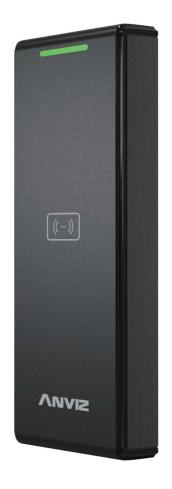
The C2SR device is a IP65 water- proof card reader, suitable for outdoor applications. It operates at 32-Bit High Speed CPU, supports 125KHz EM card or 13.56MHz mifare. The C2SR has Weigand 26/34, with operating temperature of -20°C~65°C and operating humidity of 20%-80%.
