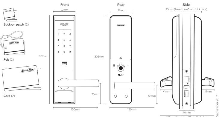
180mm (based on 40mm thick door)
